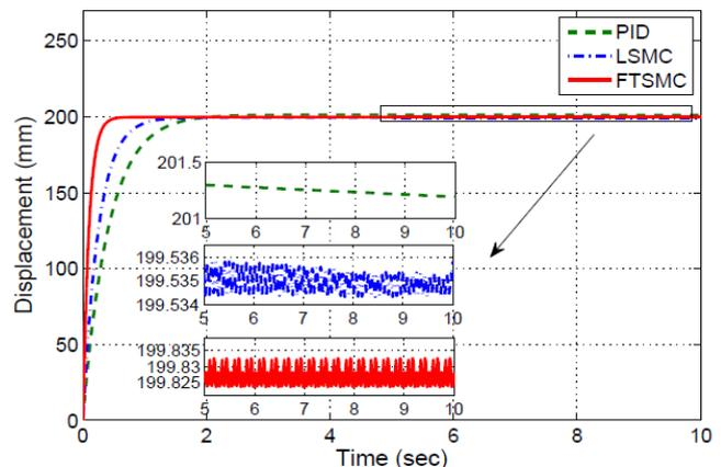
Fig. 2: The response curves for PMLM's displacement under step response in the absence of disturbance compensation.
