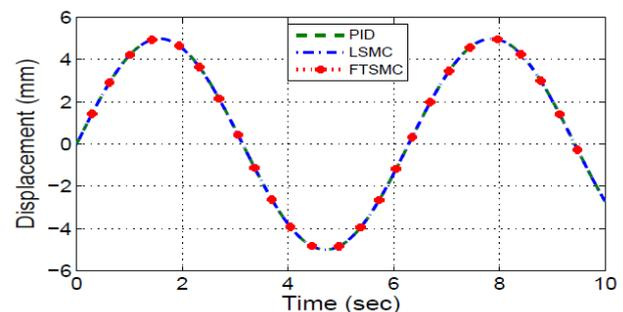
Fig. 3: The response curves for tracking a sinusoidal signal In the absence of disturbance compensation, (a) displacement, (b) Displacement error.
