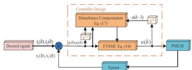
Fig. 1: The block diagram of the discrete-time FTSMC for PMLM.
