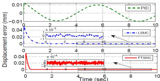
Fig. 5: The response curves for tracking a sinusoidal signal in the presence of disturbance compensation, (a) displacement, (b) Displacement error.
